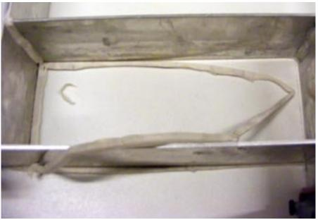
The box pressed lightly into the clay and the excess inside cut.
