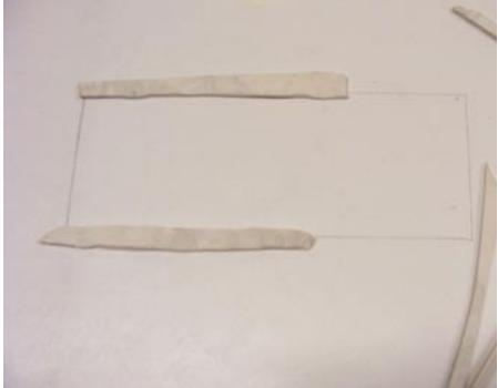
As a sealant, I use modeling clay, which I first rolled out and then I cut strips out. They are laid on the line all the way around.
